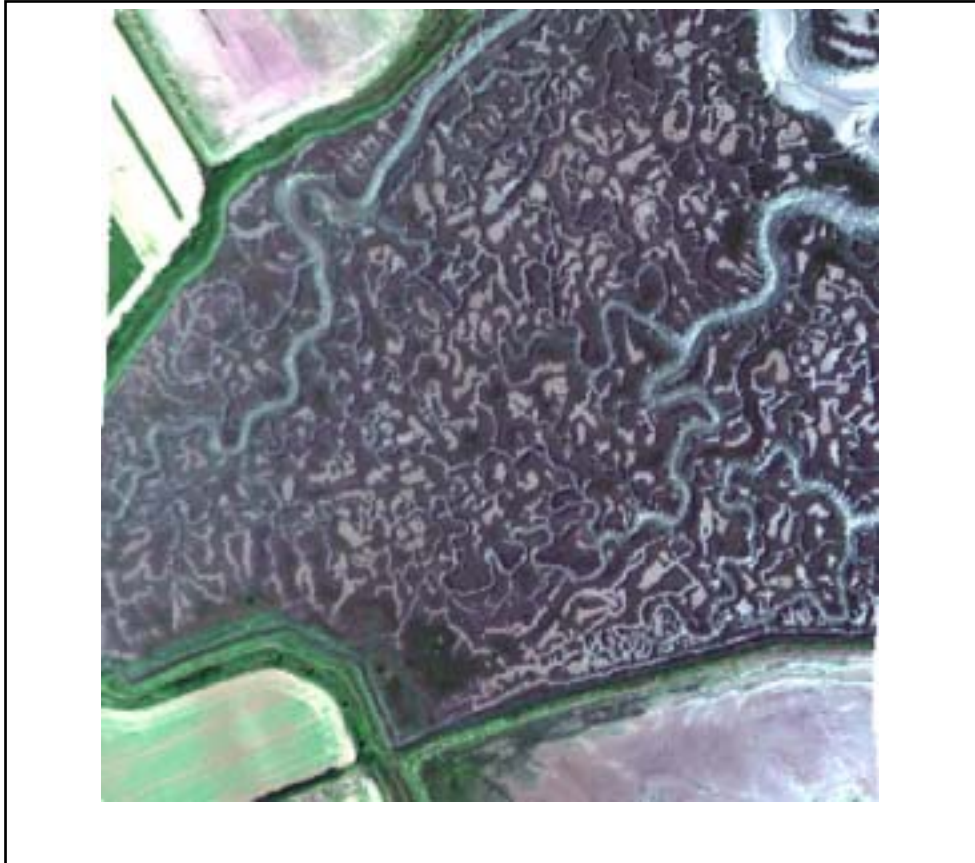
Figure C.6 Bi-directional effects in CASI imagery (Left hand edge of image: vegetation- high radiance, mud-low radiance Right hand edge of image: vegetation- low radiance, mud-high radiance)
