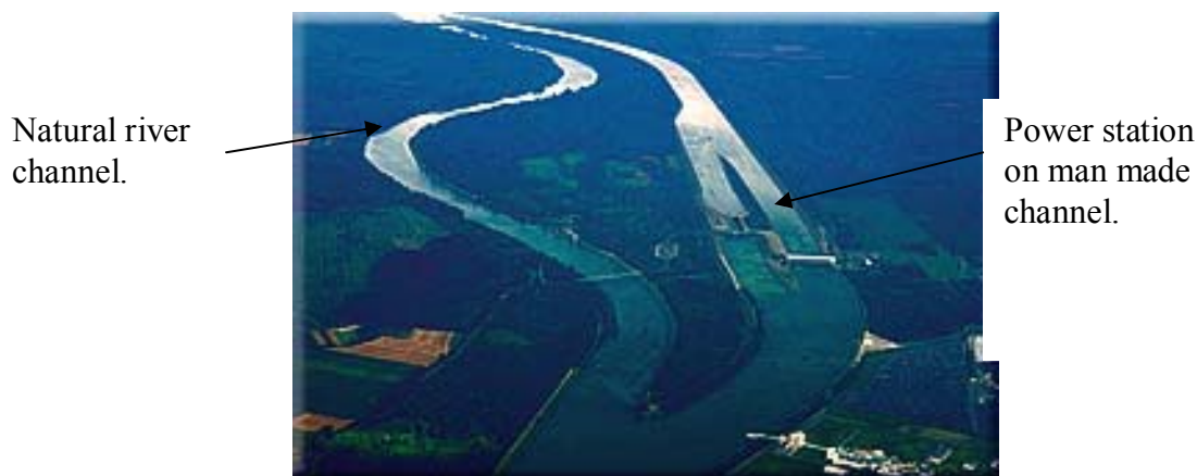
Figure A3.2 Image demonstrates the layout of a river retention scheme (Integrated Rhine Programme website, 2003)
