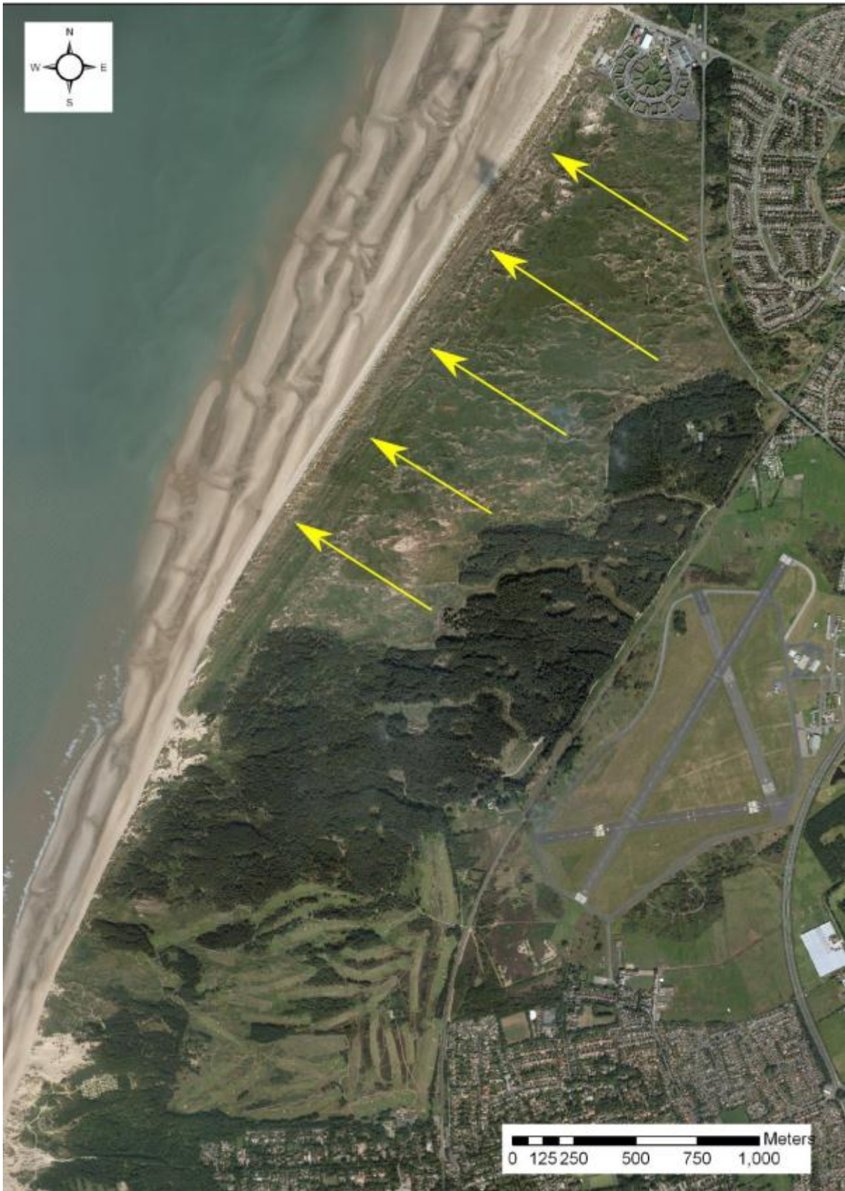
Figure 6. Ainsdale NNR and Ainsdale LNR conceptual groundwater flow diagram. The yellow arrows indicate the direction of groundwater flow. © NERC (CEH) 2013, © Next Perspectives.
