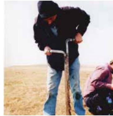
Figure 3. A one-metre long, stainless steel peat cutter for field sampling, adapted from one found at Lindow Moss that was used by hand peat-cutters (Lageard et al., 1994).
