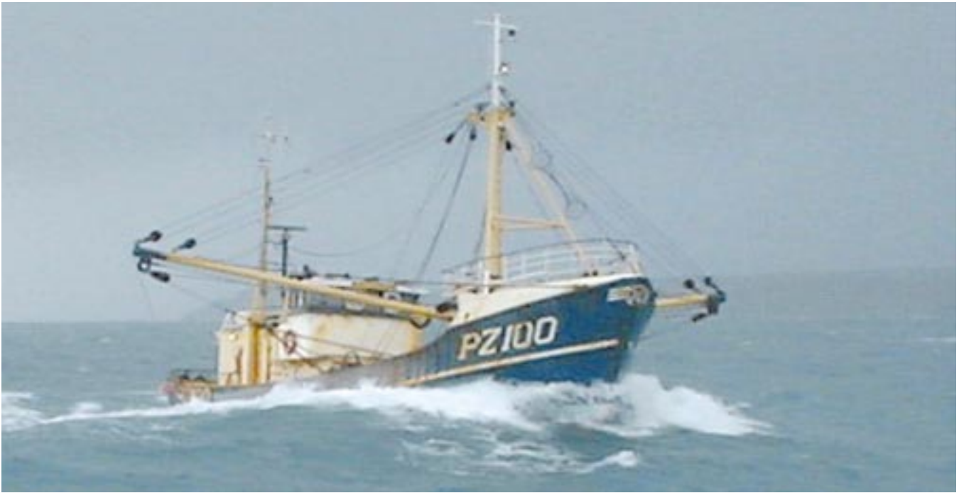
Beam trawler en route to Mounts Bay. Beams are towed from 'derricks' at right angles to the boat. Spike Searle (above)
