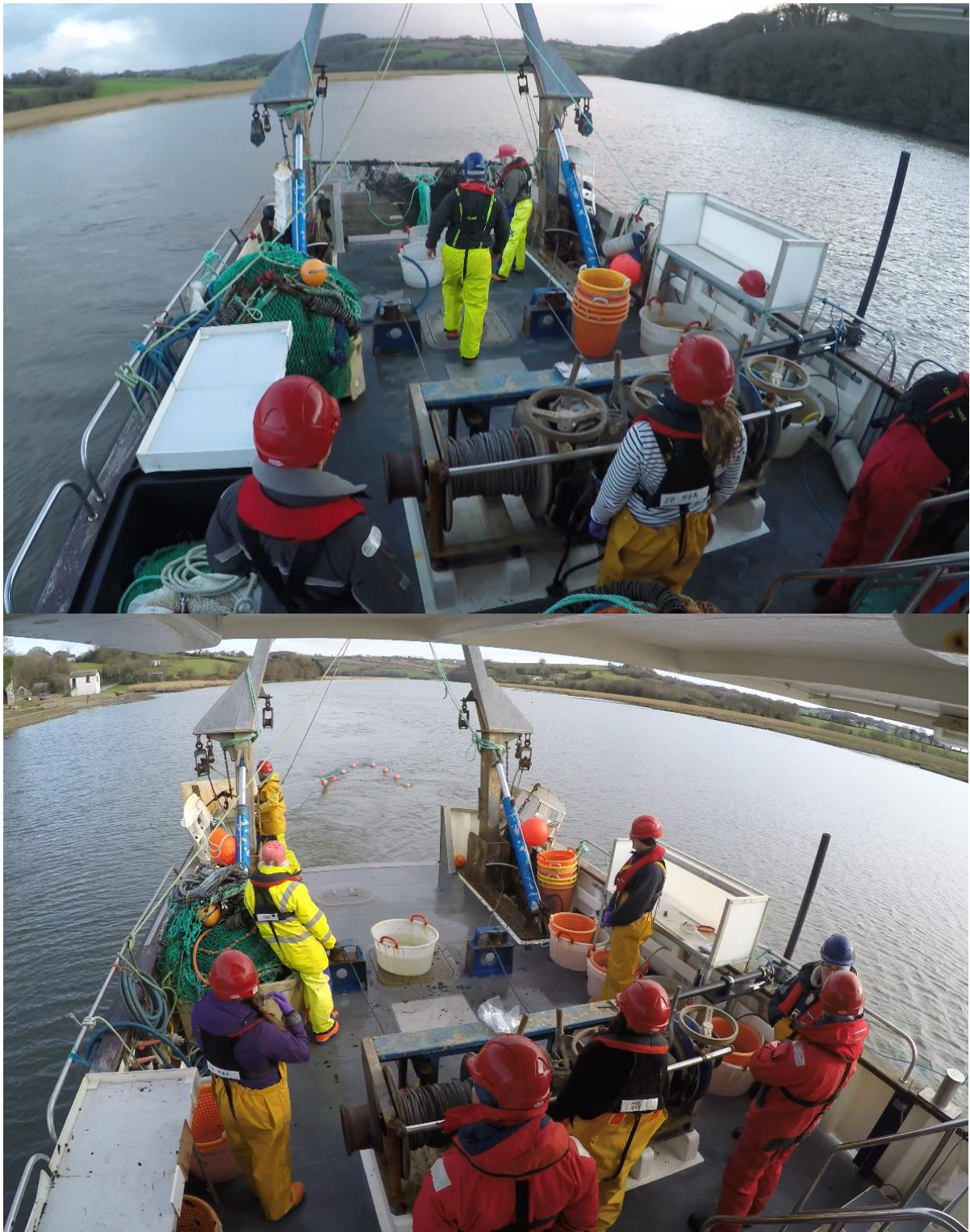
Figure 14. Example fishing gear arrangements on RV MBA SEPIA. Top, rigged with the 4m beam trawl just before deployment. Bottom, hauling the 8 fathom otter trawl with the floats on the surface. Both show two sample processing stations, the top of the SVP pole arrangement and various tubs (see text for details).
