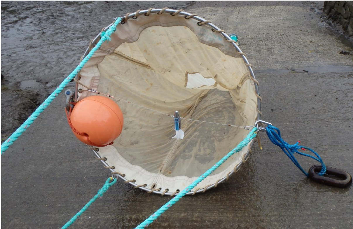
Figure 1. Plankton net laced to a 1m diameter circular, stainless steel net ring. Also shown are the 3 bridles, the top float (that would be situated outside the net), the lower weight and the mechanical flowmeter.
