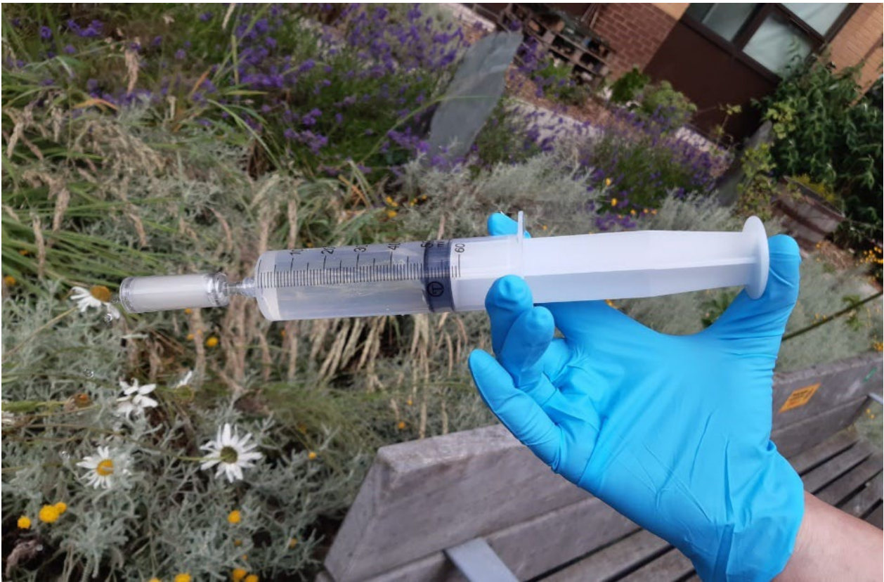
Figure 1: Syringe attached to filter (one of the 3 methods to be used in this study).
