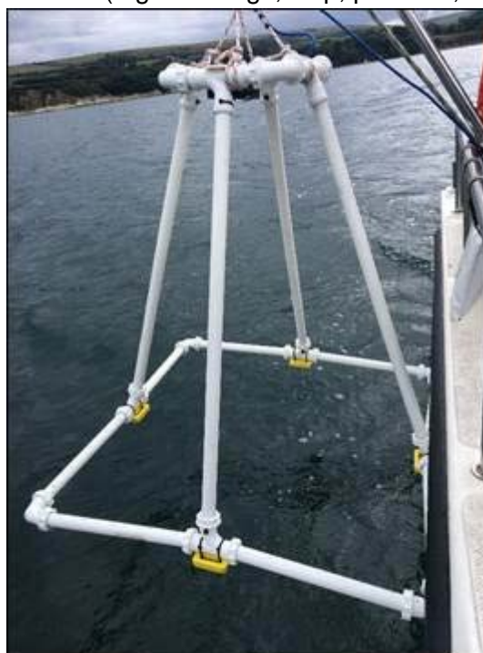
Fig. 2. DDV camera and quadrat frame being deployed from the side of the survey vessel.
