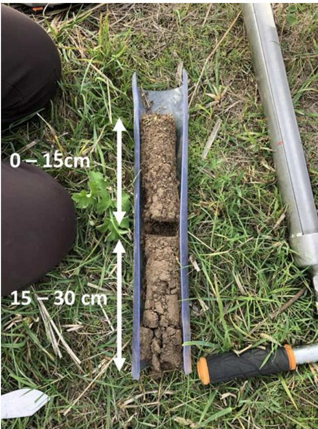
Figure 10. Example of the soil core split into the top 0 to 15 cm and bottom 15 to 30 cm before putting into sample bags. Photo credit: Becky Davess
