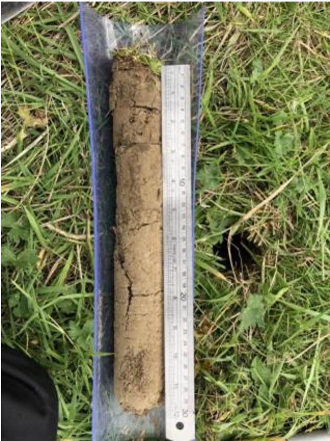
Figure 9: An extracted soil core with the intact core measured. Photo credit: Becky Davess
