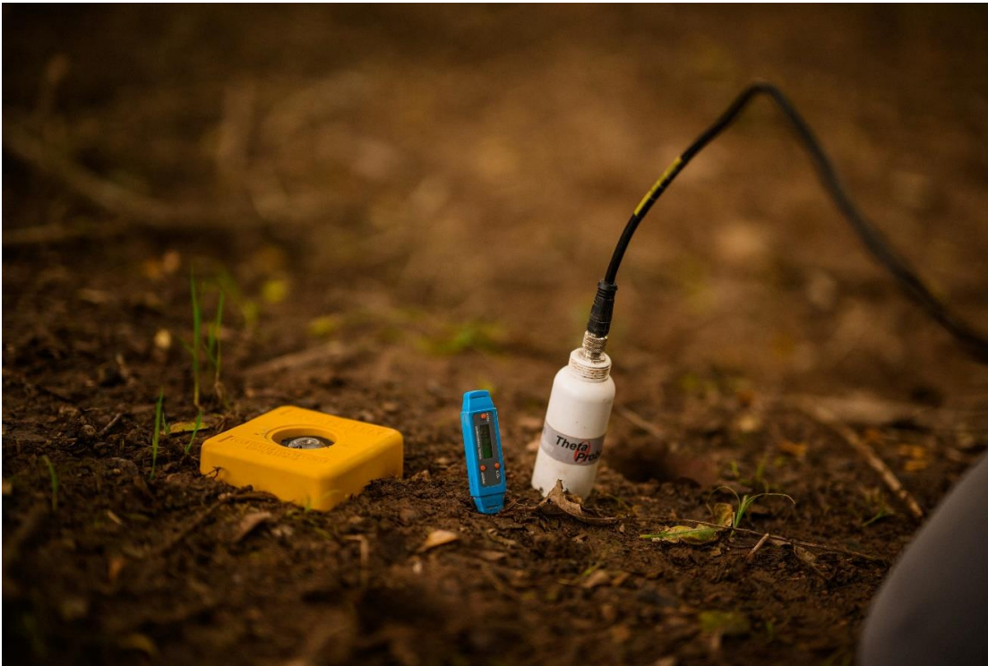
Figure 7. Example of a plot marker and the soil temperature and moisture probes. Photo credit: Chris Parkes
