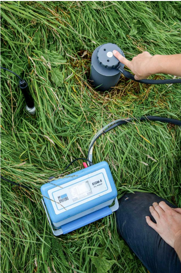
Figure 13. Left: PP Systems EGM-5 Gas Analyser and SRC-2 Soil Respiration Chamber. Right: PP Systems SRC-2 Soil Respiration Chamber and CPY-5 Net Canopy Chamber. Photo credit: Celina Jennings
