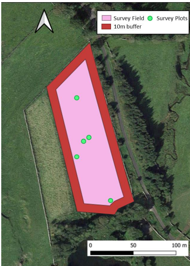
Figure 1. Example of random plot selection for soil coring and vegetation surveys, made with QGIS.
