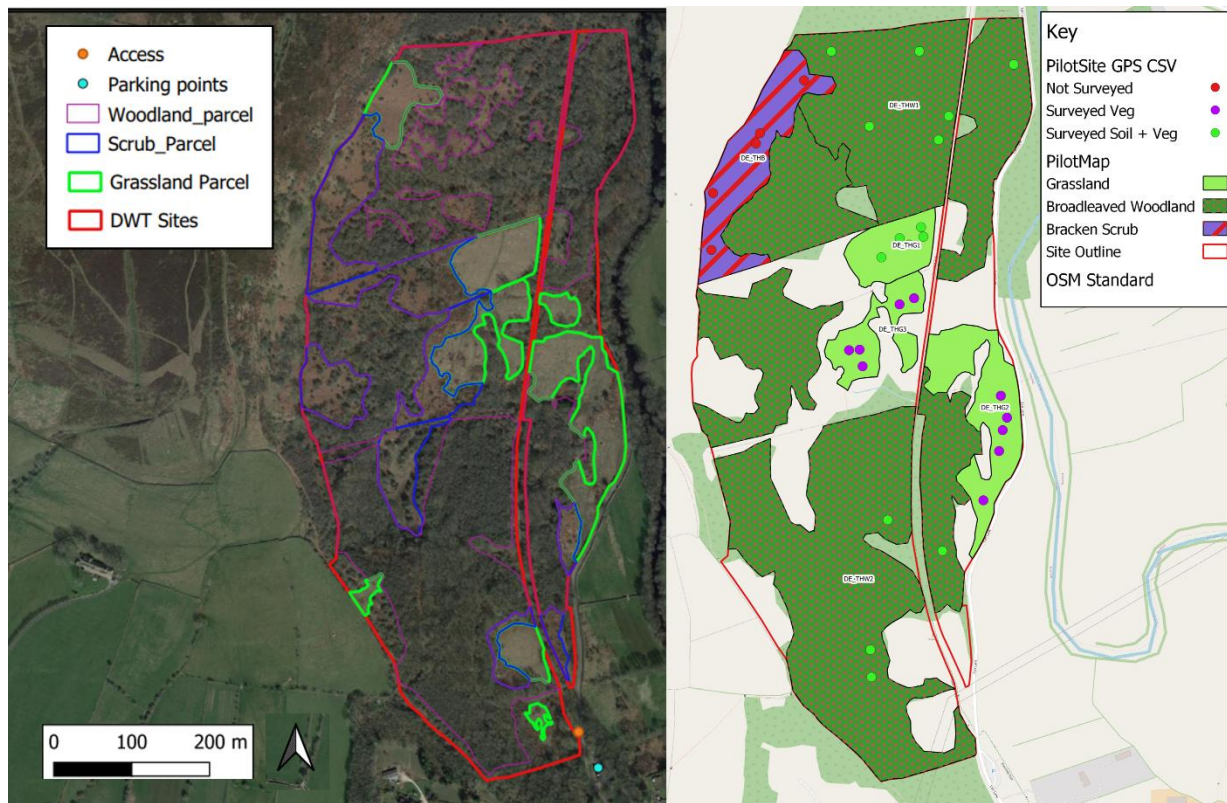
Figure 3. Left: Map of Thornhill, Derbyshire Wildlife Trust, with a mix of different habitats including grassland, scrub and woodland. Polygons are drawn round the different habitats in QGIS. Right: Map of the same area showing the land parcels attributed to the different habitats identified on the left and 5 random plots are generated within each parcel, made with QGIS.
