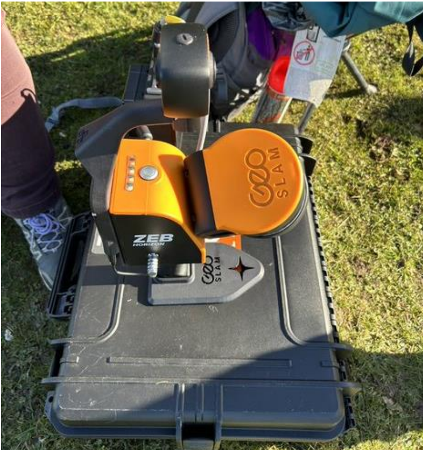
Figure 26. The Faro ZEB-Horizon 3D laser scanner. Photo credit: Becky Davess
