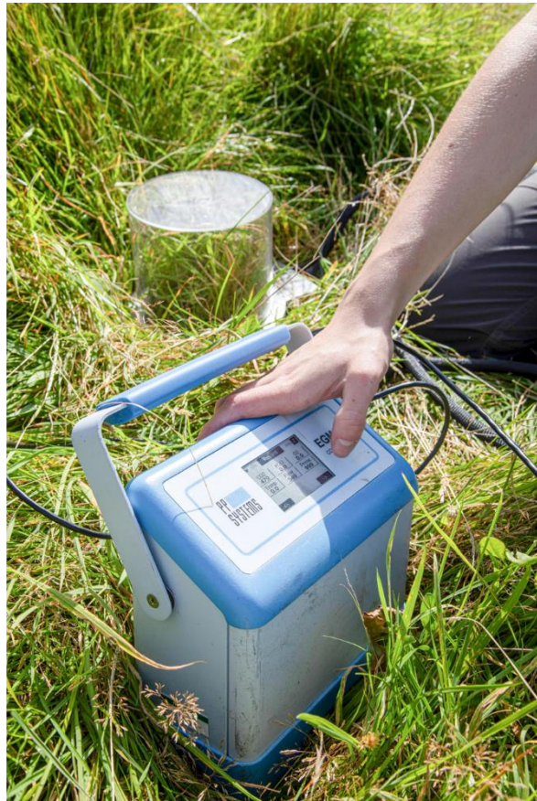
Figure 13. Left: PP Systems EGM-5 Gas Analyser and SRC-2 Soil Respiration Chamber. Right: PP Systems SRC-2 Soil Respiration Chamber and CPY-5 Net Canopy Chamber. Photo credit: Celina Jennings
