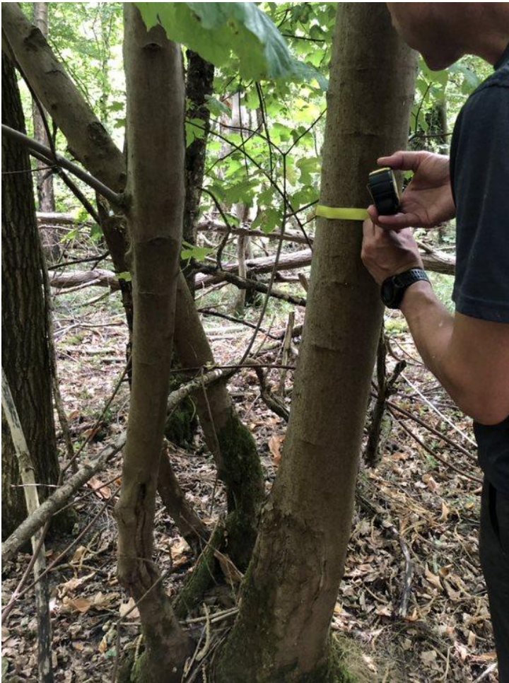
Figure 16. Measuring the diameter at breast height (DBH) of a tree with a diameter tape. Photo credit: Tamsin Lockwood
