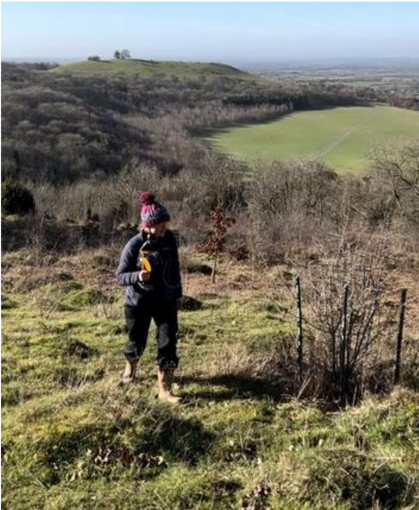
Figure 27. Walking around the scrub in continuous closed loops for approximately 20 minutes holding the ZEB-Horizon 3D laser scanner. Location: Coombe Hill National Trust, Buckinghamshire. Photo credit: Mandy Cooper
