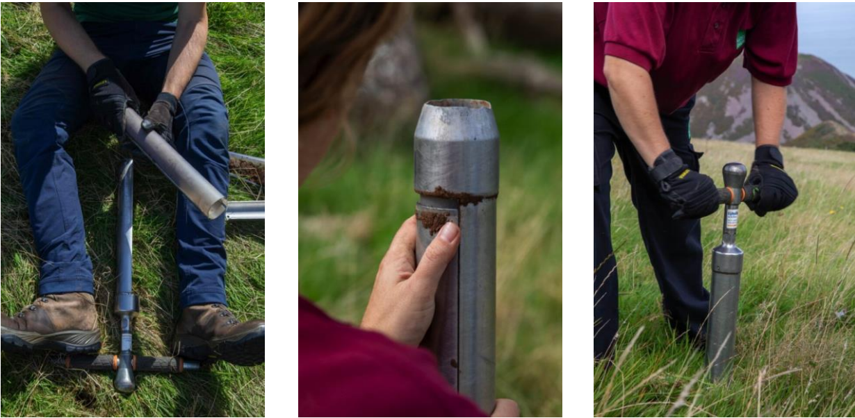
Figure 6. Assembly of the soil corer. Left to right: The transparent liner is inserted into one half of the corer; the corer is slotted back together with the liner inside and is fixed with the locking pin. The coring location is identified, and sample collection is ready. Photo credit: Celina Jennings
