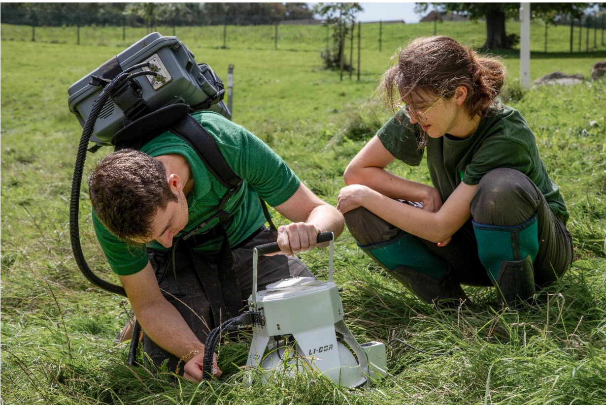
Figure 14. Licor-7810 trace gas analyser for measuring methane. Photo credit: Celina Jennings
