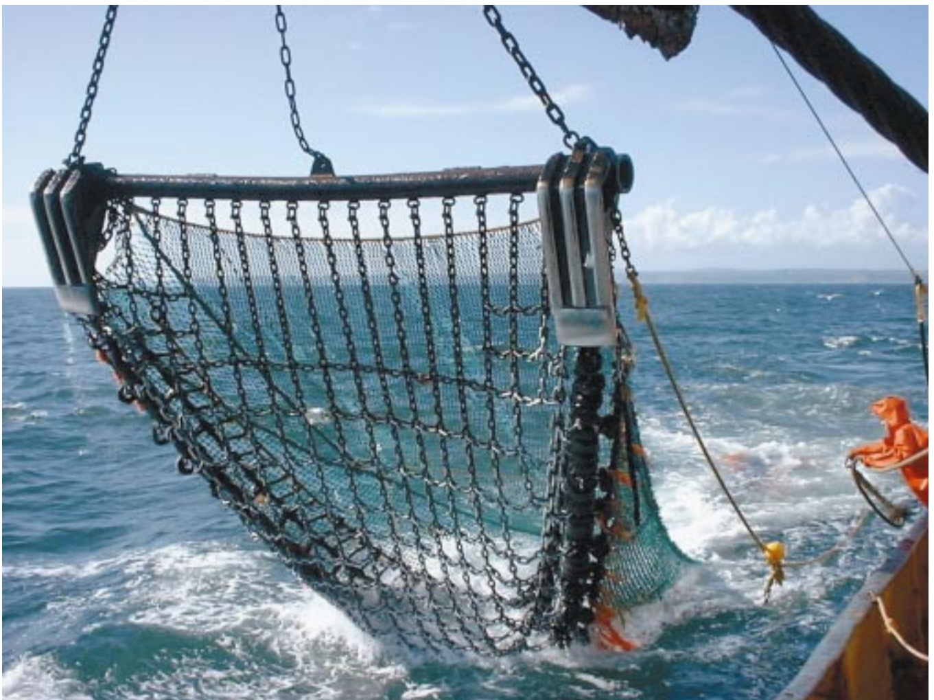
Hauling in a beam trawl, showing the skids enabling the net to be trawled on the seabed. Spike Searle
