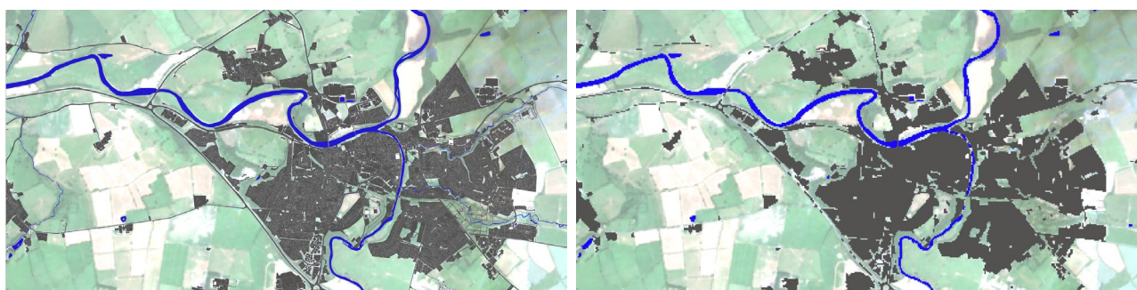
Figure 6: Comparison between raw OSMM data (left) and the processed segments used in Living England 2022-23 (right) to inform ‘Built-up Areas and Gardens’ in black and the ‘Water’ in blue.
