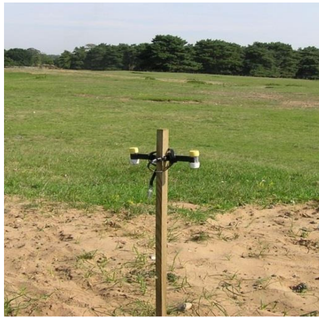
Figure 2.1 Nitrogen diffusion Tubes attached to a sample post 1 m above ground level (from Lambert and Davy 2011).
