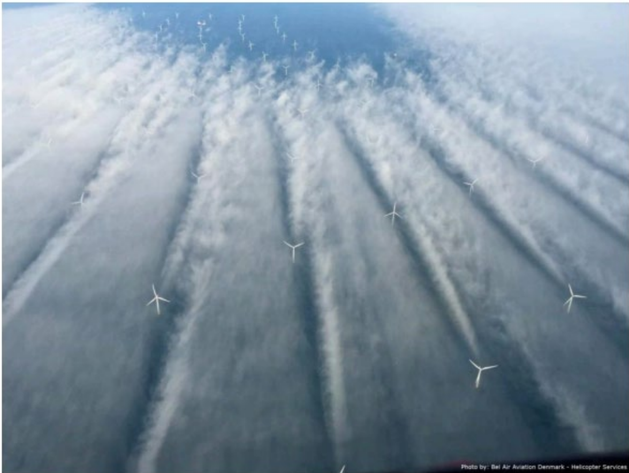
Figure 4-1. Photograph of the wind wake effect at Horns Rev II wind farm (Hasager et al. , 2017)
