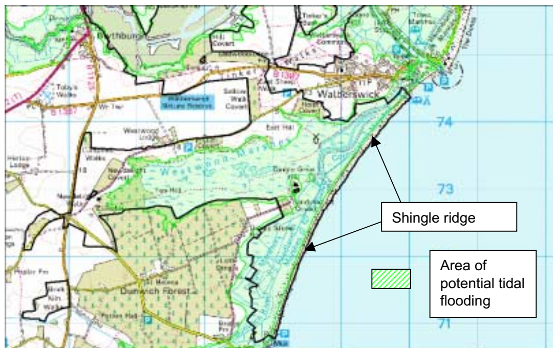
Figure 4.2 Westwood Marshes and extent of tidal flooding that could occur following significant breach and breakdown of the fronting shingle ridge.
