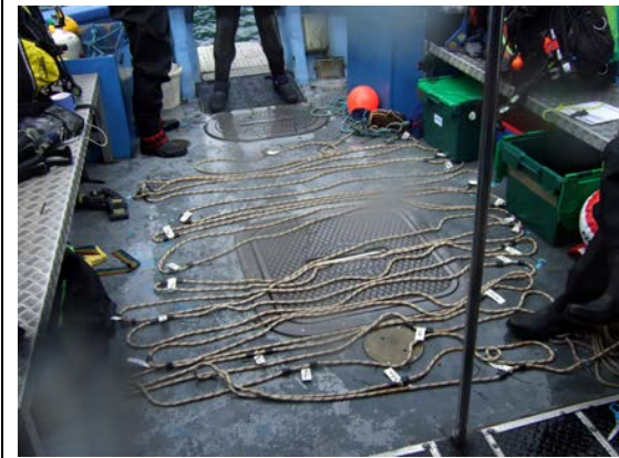
Plate 3. 50 m sinking line on the aft deck, with marker tags at 2 m intervals. Photo by Chris Pirie.
