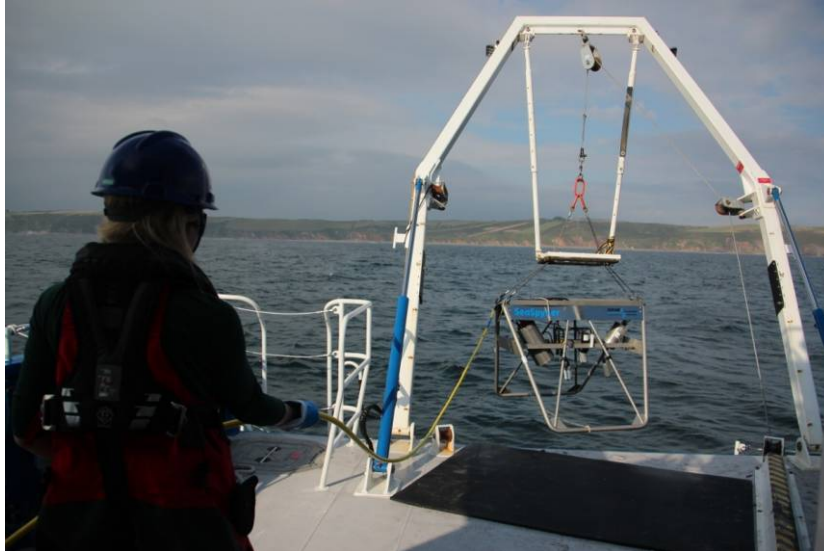
Figure 4. STR SeaSpyder Drop Camera system being deployed from the stern of the coastal survey vessel.
