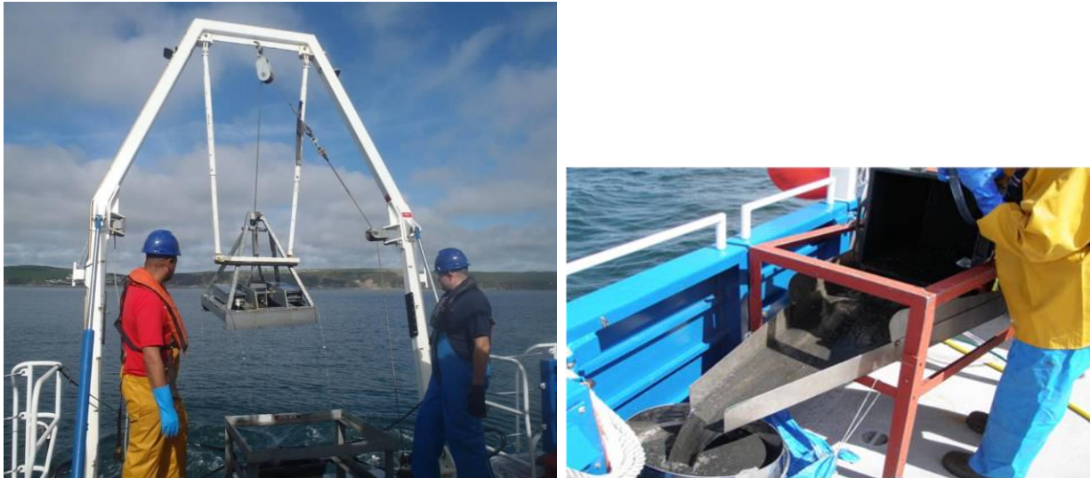
Figure 4. Mini-Hamon grab (left), and equipment for sieving benthic fauna samples (right)
