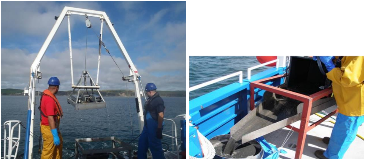
Figure 6. Mini-Hamon grab (left), and equipment for sieving benthic fauna samples (right)
