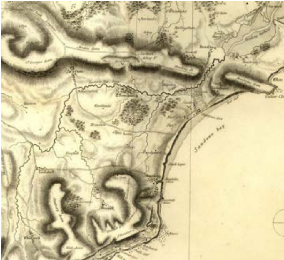
Fig. 6.10: This map of the Isle of Wight by Sir Henry Englefield (1816) shows the extent of the Eastern Yar catchment, emerging as springs from the Gault Clay spring line behind Wroxall and Whitwell, before joining to cross the Arreton Valley, and then subsequently forming a cutting through the Chalk Downs to emerge at Brading Harbour. Private Collection.
