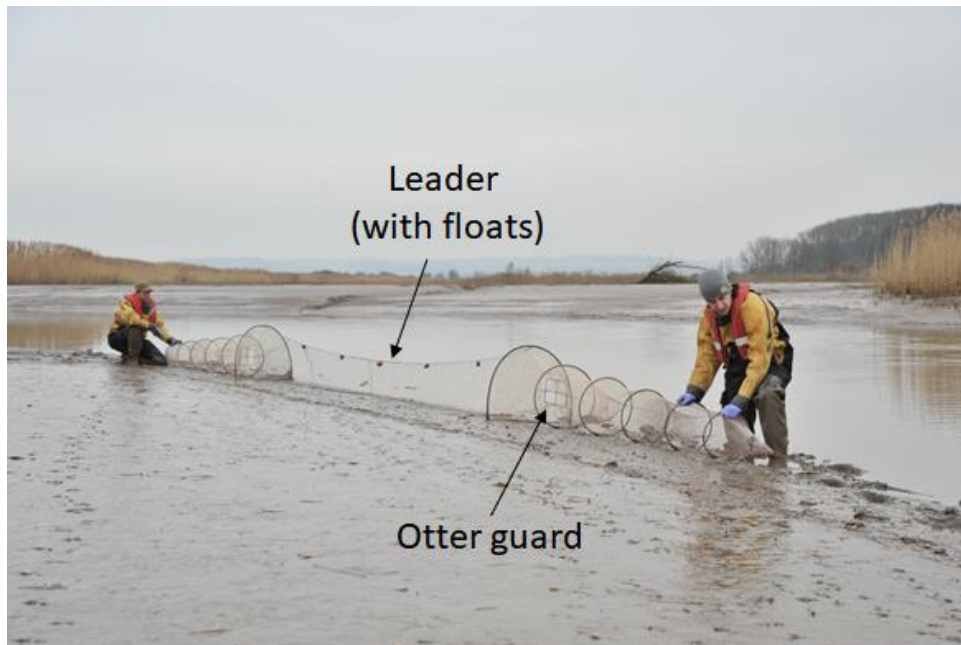
Plate 2. Deployment of the paired Dutch 'D' type fyke net in an intertidal area of the Humber Estuary. Photo by University of Hull.
