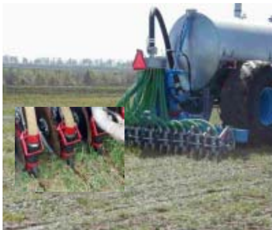
Figure 2. Slurry spreading techniques to reduce ammonia volatilisation.
