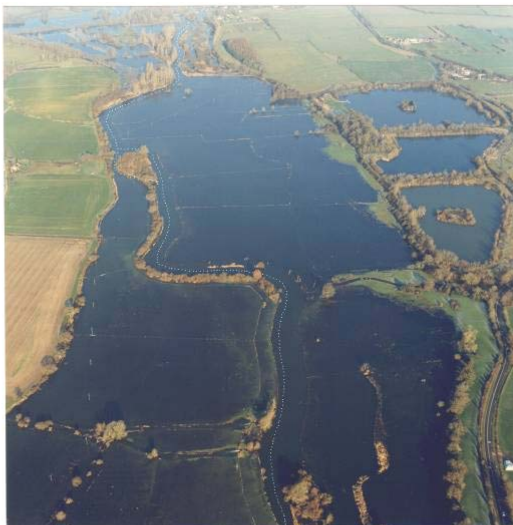
Figure 6.1. Aerial view of the flooded valley upstream of Ibsley Bridge, January 5 2003. This view is looking North (upstream), with Ibsley Bridge off the bottom of the picture, and Bickton at the top. The white dotted line indicates the approximate centre-line of the river. Note that the West bank of the river is higher than the fields behind it, probably as the result of dredging spoil dumped on the bank. In the centre foreground the two hatchpools on side stream leading to the Harbridge Stream are visible. In the middle right the Huckles Brook enters across a raised delta, created by gravel being washed down the stream. Most of the trees on the floodplain are along the banks of the main river and side streams. Photo by Stills Photography, on behalf of the Environment Agency.
