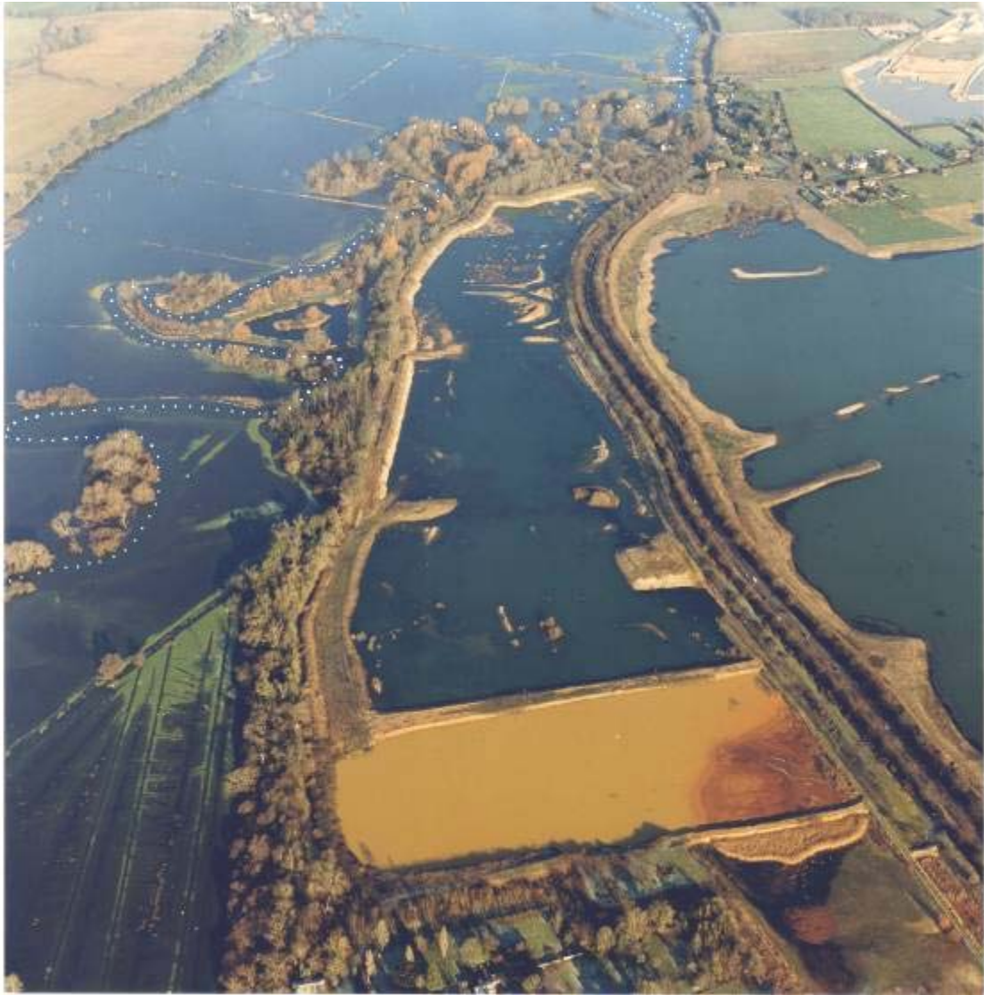
Figure 6.2. The next river reach downstream from Figure 4.1 taken on the same day, with Ibsley Bridge near the top of the picture. The white dotted line indicates the approximate centre-line of the river. Note again that most of the trees and scrub in the floodplain are along the river. Also note that the watermeadows in the left foreground are higher than the flooded area of the valley. Photo by Stills Photography, on behalf of the Environment Agency.
