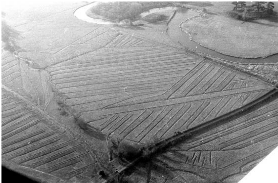
Figure 6.3. Aerial view of the watermeadows at Ellingham, December 1986. The picture is taken looking SW, with Ellingham Drive in the foreground. The lower part of the Ellingham Carrier (Channel 6.5.1) runs close to the river, and the gently-curved Woodside Carrier (Channel 6.5.2) and the more sinuous Woodside Drawn (Channel 6.6) can be seen on the left. The low angle of the sun shows up the individual channels well. Some grazing swans can be seen on the right centre but it is not known if they were mute or Bewick's.
