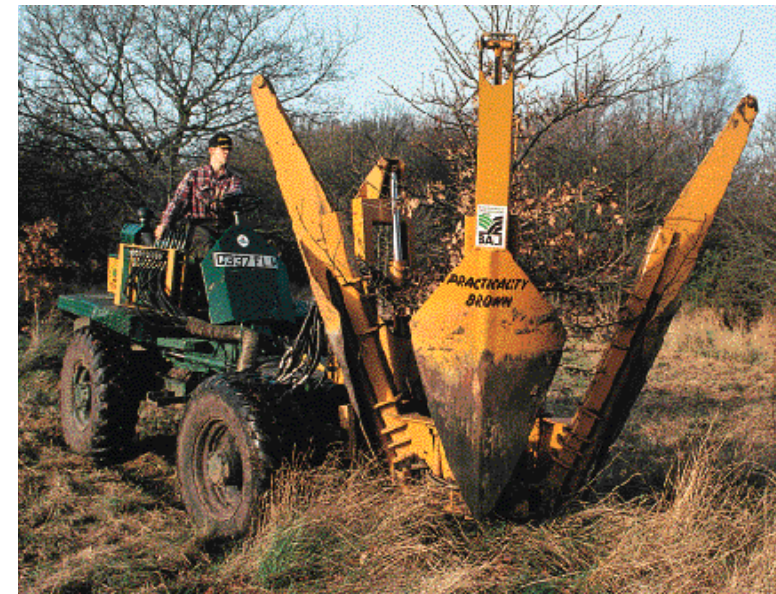
Figure 44a. A treespade being used to move a young oak tree at Ashted Common (Surrey),
